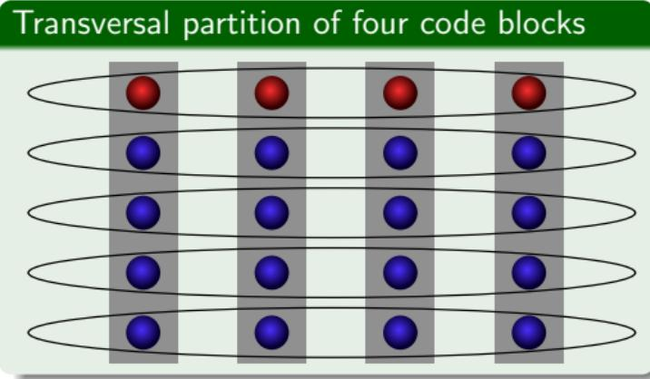
Transversal gates are fault tolerant because each code block is corrected independently.
