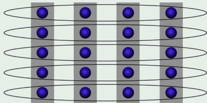
Transversal gates are fault tolerant because each code block is corrected independently.
