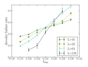
$\hookrightarrow$  threshold at  $t_{sim} \simeq 0.125$
